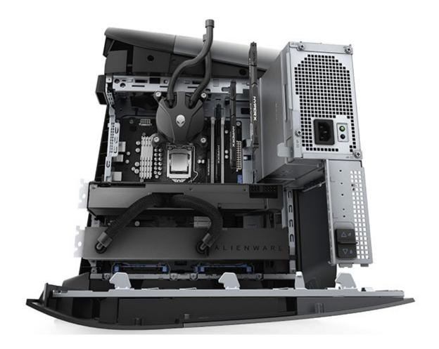
Described as an industry first by the company, the Rad Card enables a liquid-cooled GPU in a smaller chassis while allowing enough space for a liquid-cooled CPU in the same case. The result, Asetek says, is superior cooling over an air-cooled system, ensuring GPU stability and limiting thermal throttling. In addition, the design eliminates the clutter of tube routing, making for a clean and sparse system environment.
