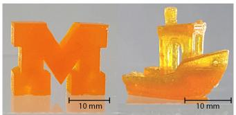
The light-based system literally lifts complex objects from a vat of liquid. To do so, the researchers use two lights to control where the resin hardens and where it remains fluid, allowing them to solidify the resin into more sophisticated patterns. The creation of a regions with no solidification allows the use of thicker resins (potentially with strengthening powder additives) for the production of more durable objects.
