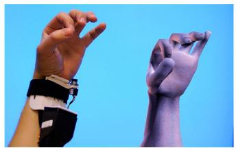
Dubbed the "Digits Project," the wrist-mounted device takes some inspiration from the Kinect. Using diffuse infrared light, IR laser, camera and inertial measurements the system software builds a 3D model of the moving hand the researchers claim is accurate to within one hundredth of a centimetre.
