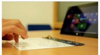
The surface is both lightweight and flexible, meaning OEMs can integrate it into protective covers or provide larger desktop touch zones. It can also act as a super-slim keyboard or detect handwriting or sketches via modified pen, with touch latency of just 12 milliseconds.
