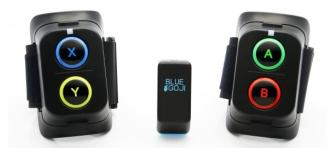
The Goji Play system consists of two controllers and a wearable motion tracker. Each controller features 2 buttons and attaches to fitness equipment handlebars via velcro straps, while the tracker clips to belts or simply slips in users' pockets.
