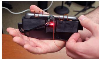
"This is the first gesture recognition system that can be implemented for less than a dollar and doesn't require a battery," UW assistant professor Shyam Gollakota says. "You can leverage TV signals both as a source of power and as a source of gesture recognition."
