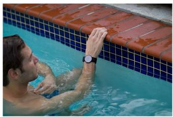
Made by a ex-Apple engineer Nikola Hu and Microsoft Research sensor expert Meng Li, the Moov uses gyroscopes, accelerometers and magnetometers to analyse body movements in 3D. Thus, the makers claim, the device actually acts as a "virtual coach," providing tips according to wearer performance.
