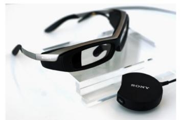
According to the company the lenses are 85% transparent, 3mm thick and act as a monochrome display, allowing for higher brightness and lower energy consumption. Meanwhile the frames pack an array of sensors, including a 3MP camera, accelerometer, gyroscope, compass, brightness sensor and a microphone.
