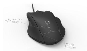
The sensors measure heart rate, galvanic skin response and actions per minute, and QG software plots gathered data in a series of graphs. Users can view the data as a transparent on-screen overlay during gameplay, one complete with real-time feedback such as threshold warnings. You know, in case one needs to be reminded to take a break from too much CounterStrike...
