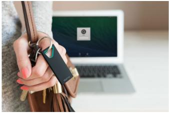
The Sesame 2 is a wireless sensor small and light (10g) enough to attach to a keychain or keep in a pocket. It pairs with OS X machines via Bluetooth 4.0 and companion Sesame app, and handles a number of security features, such as the aforementioned automatic locking and optional 2-factor authentication demanding the use of both Sesame 2 and a password.
