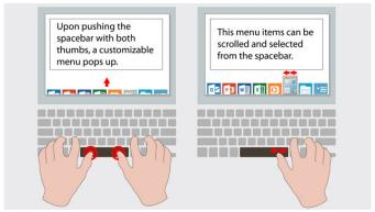
The SpaceBar essentially turns the space bar into a touch-sensitive surface complete with customisable gesture controls, such as thumb swipes (for word selection) and touchscreen-style double-thumb pinch zooming. Also included are 5 "logical buttons" users can program via macro editor to provide further shortcuts for desktop functions or game controls.
