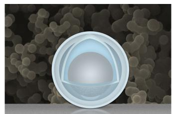
The "egg" in question consists of an aluminium nanoparticle (the "yolk") surrounded by a titanium dioxide (aka titania) "shell." According to the researchers the combination is a "high-rate champion among high-capacity anodes," meaning it can lead to the more powerful batteries of the future.
