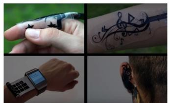
The iSkin consists of biocompatible silicone rubber (specifically polydimethylsiloxane, aka PDMS) and conductive carbon black powder. It carries multiple pressure-sensitive sensors and is flexible enough to detect input pressure even when stretched by up to 30% or bent at a radius of 0.5cm.
