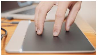
The Morph carries 20000 pressure sensors allowing to detect and measure even the slightest of touches. It is non-capacitive, allowing one to use it with objects such as a paintbrush as well as their fingers.
