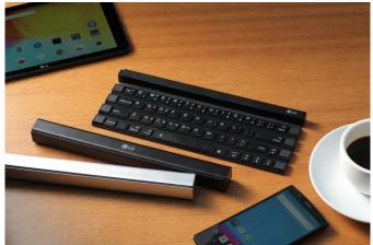
The Rolly Keyboard features a 17mm key pitch (most desktop keyboards have 18mm pitch) with "satisfying" tactile feedback. Construction is in polycarbonate and ABS plastic, and a pair of foldable arms smartphones and tablets in an upright position.
