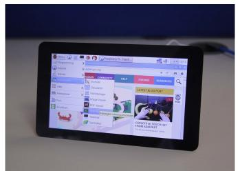
Based on an industrial-quality Inelco Hunter display, the touchscreen is a 7-inch 800x480 resolution number offering 10-point capacitive touch input. It connects to the Raspberry Pi via DSI (display serial interface) connector, allowing users to connect a second monitor via HDMI port.
