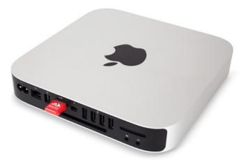
The adapter fools the Mac mini into thinking a display is attached, meaning video drivers are loaded and GPU is fully activated for 100% full video performance, with no choppy images or mouse lag.
