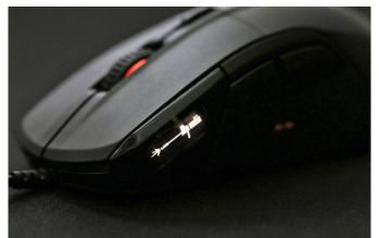
First seen back at CES 2016, the Rival 700 carries what SteelSeries describes as a "tactile engine" providing users with customisable vibrating patterns, feedback durations and triggers, among others. For instance, player can set the mouse to vibrate whenever a game cooldown is over, or provide a heartbeat-like sensation when health is low.
