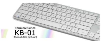
Both keyboards feature chiclet-style keys backed with scissor switches arranged in a standard 104 key layout complete with combo media keys and LEDs for num lock, caps lock and battery level. The underside of the keyboards houses power and pairing buttons together with rubber non-slip feet and flip-out rear stands.
