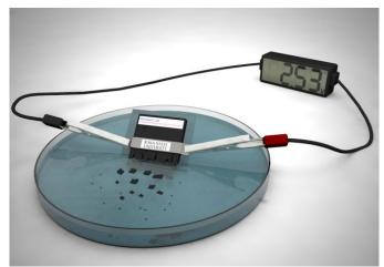
Developed by Iowa State University, the battery is designed to power so-called "transient electronics," devices able to perform a variety of functions until exposure to light, heat or liquid. An obvious application for such devices is the military and espionage, but these also find use in medicine (specifically implants able to melt away when no longer needed) and temporary environmental sensors.
