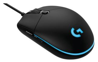
Designed for eSports athletes, the G Pro follows on the company's previous G100s and G303 rodents with a sensor covering the entire DPI range (200-12000) with zero smoothing, filtering or acceleration for "exceptional" tracking accuracy and responsiveness. The buttons are also improved, as a metal spring tensioning system reduces the force required to click while ehancing consistency.
