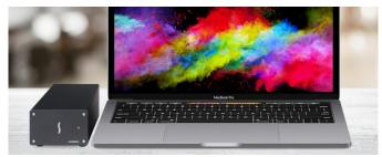
The SEL and SE I are compact single-slot expansion systems taking advantage of the 2750MB/s PCIe bandwidth offered by Thunderbolt 3. The SEL is the smallest of the two, and houses one low-profile single-width PCIe 3.0 card, such as Thunderbolt-compatible 16 and 8Gb fibre channel, 40 and 10Gbps ethernet, 6Gbps or 12Gbps SAS and host bus adapters, RAID controller cards and even low-profile pro video capture cards like the BlueFish 444 Epoch 4K Neutron.
