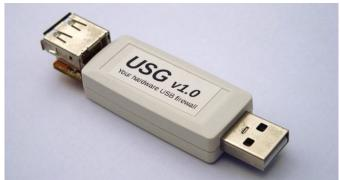
BadUSB is a sinister piece of malware able to bypass the OS, antivirus software and other security measures. It can attack by hopping into PCs through the USB port, for example via USB sticks supplied by customers or colleagues. This lead to Fisk working on a hardware solution for access to untrusted USB devices, without need for a USB condom or disabling USB ports.
