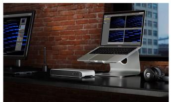
In total the dock offers three USB 3.0 ports, gigabit ethernet port, two Thunderbolt USB-C ports, DisplayPort with DisplayPort 1.2 support, 3.5mm headphone jack and 3.5mm microphone input jack. It handles either one 5K (5120 x 2880 resolution) display at 60Hz via Thunderbolt 3 port or two 4K (4096 x 2160) displays simultaneously at 60Hz using the DisplayPort and Thunderbolt 3 port.
