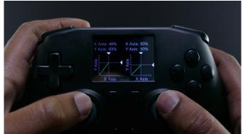
The All Controller is similar in design to the Xbox One controller, if with a small display set in the centre. The makers claim it works with a wide range of machines, including PS3, PS4, Xbox 360, Xbox One, Switch and Wii U, as well as PCs, Macs, iDevices and Android devices. This variety of compatible hardware is where the display comes in, since it allows users to set up the controller accordingly.
