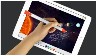
The Crayon borrows technology from the Apple Pencil with the smart tip allowing users to adjust line weight according to the angle. It does not offer pressure sensitivity, but does include palm rejection technology and MFI-certified charging through built-in Lightning port. Logitech says a single charge allows for up to 7 hours of use.
