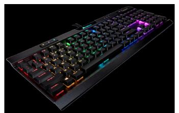
According to the company the Cherry MX Low Profile keyswitches offer the same performance as regular Cherry mechanical switches with a lower 11.9mm height and short actuation distance. Combined with redesigned low profile keycaps the switches reduce the full keypress distance to both bottom out the key and actuate the switch, lessening keypress fatigue.
