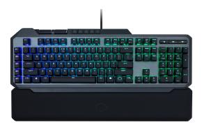
Dubbed "Aimpad," the technology adds IR sensors to the Cherry MX switches in the QWERASDF key cluster. According to Cooler Master, the IR sensors "sense the entire 4mm range of a key press versus competitor analogue keyboards that are only capable of measuring 2mm of analogue movement and do not utilize Cherry MX switches." Or, in short, the pressure sensitivity allows for smooth increments in the control of speed, yaw, pitch and the like, similar to what is offered by analogue joysticks.
