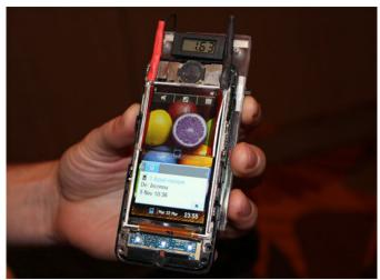
Wysips proposes a means to eliminate chargers of any kind-- by turning device screens into solar chargers.
