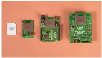
Created by ex-Apple and Google engineers, the Electric Imp card looks very similar to standard SD cards. It carries a wifi 802.11b/g/n radio, a Cortex M3-based processor and software-controllable I/O pins.
