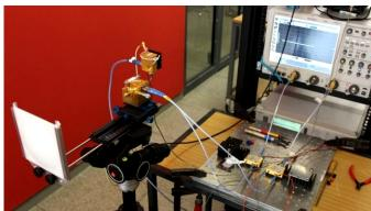
The wifi tests use 237.5GHz signals over a distance of 20m in laboratory conditions. However the super-high frequencies involved demand clear line of sight between devices at all times.
