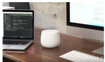
According to the makers the device is fairly easy to use, as one simply needs to connect it to the router before setup via companion app. Once installed the Cujo scans incoming traffic for potential threats such as intrusions, malware and viruses.
