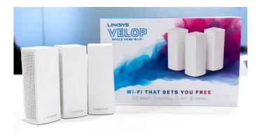
The Velop system uses a tri-band 802.11ac MU-MIMO mesh network, with one band dedicated to communication between routers to prevent some of the bottlenecks two-band systems suffer from. The routers also include two ethernet ports in case customers prefer cable connectivity. The mesh system is self-healing, and can handle up to 5 Velop units to ensure wifi coverage in even the largest of houses.
