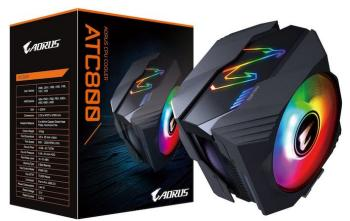
Reaching inside the aluminium fans are six direct contact nickel-plated copper heatpipes. A plastic shroud covers the fans and the top of the cooler. The top features an RGB-lit Aorus logo and a temperature/RPM reader, and the fans are also full RGB. All lighting can, of course, be synchronised via Gigabyte motherboard software.
