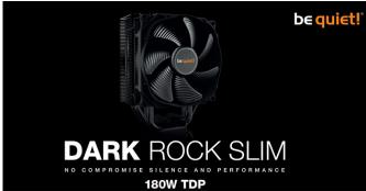
The Dark Rock Slim measures 72 x 127 x 159.4mm, meaning it requires a chassis with clearance of 160mm or more. It features a cooling block with airflow-optimised cooling fins to increase air circulation, and further improves on heat transfer through a black coating with ceramic particles and four 6mm copper heatpipes. The top cover is in brushed aluminium with a diamond cut finish.
