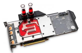
Thanks to a switch to a 7nm fabrication process, the Navi GPU cores inside the RX 5700 and 5700 XT are 251mm in size (compared to the 495mm Vega GPUs). The reduction in size makes for a more efficient GPU, but also increases thermal density, bringing the need for an efficient cooling solution. EK says the water blocks directly cool the GPU, memory and VRM (voltage regulation module), channeling liquid cooling directly over these critical areas.
