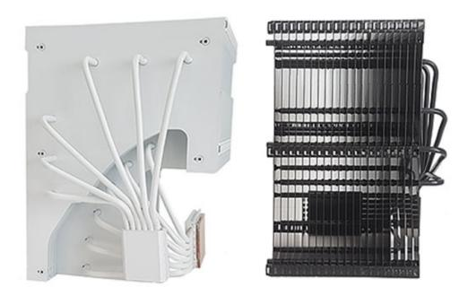
The Heart is possibly one of the biggest PC coolers around, measuring 200 x 185 x 265mm and weighing 3kg. As one might imagine it does not fit inside regular PC cases, being designed around the aforementioned The First, but enthusiast customers might find it useful for custom builds. According to MonsterLabo, The Heart can cool up to a 100W CPU and 120W GPU in a fanless configuration, and the addition of a slow-turning 140mm fan boosts the totals by 40W.
