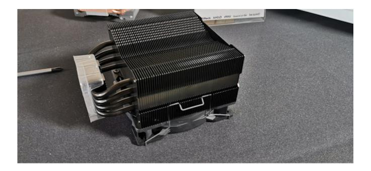
Aimed at entry-level users, the Pure Rock 2 has four 6mm heatpipes with a direct contact baseplate design for improved cooling performance. An asymmetrical design aids memory compatibility, and the package includes fan retention clips for two fans as well as the aforementioned single Pure Wings 2 120mm PWM cooling fan.
