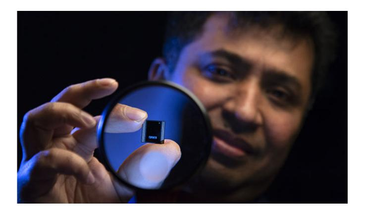
Dubbed Foveros, the process stacks components in three dimensions, making something of a silicon layer cake (if one just 1mm thick). Such packaging technology allows Chipzilla to "mix and match" technology IP blocks with various memory and I/O elements in a small physical package, allowing for "significantly reduced" board size.
