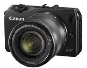
"Mirrorless" cameras lack conventional mirror-based viewfinders (using a digital equivalent) allowing for lighter, more compact bodies with the capability for intechangeable lenses.
