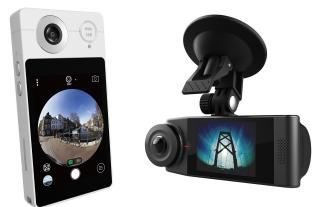
The Holo360 is the size and shape of a smartphone, and uses a Qualcomm Snapdragon 625 processor to stitch 4K resolution 360-degree videos. It features a 3-inch touchscreen and runs on Android 7.1, making it easy to share videos without need for connection to a smartphone or PC.
