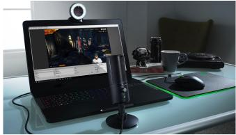
The Kiyo features an adjustable ring light with 12 white LEDs users can control to 12 levels of brightness. It has a 4MP camera able to record either 1080p video at 30fps or 720p video at 60fps, and is compatible with the XSplit and Open Broadcaster Software streaming tools. Connectivity comes through 1.5m braided USB 2.0 cable.
