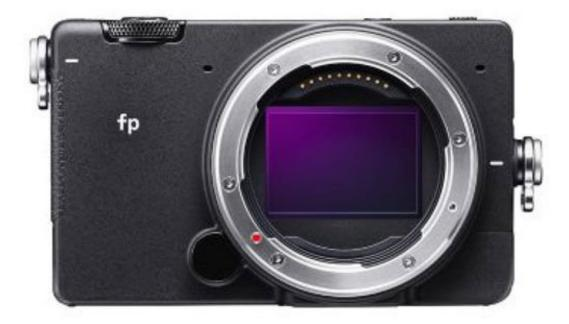
The Sigma fp measures  $112.6 \times 69.9 \times 45.3$ mm and weighs 370g (without battery or camera). Inside the die-cast compact aluminium body is a back-illuminated 35mm full-frame Bayer sensor with 24.6 effective megapixels. Construction promises to be not only robust, but also includes a built-in heatsink and is sealed in 42 points for a dust- and splash-proofing.
