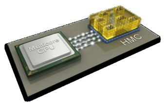
The result of a 17-month long collective effort led by Micron, Samsung and Hynix, the technology stacks multiple memory dies on top of a DRAM controller. In turn DRAM connects to the controller via silicon Vertical Interconnect Access (VIA), a technology passing a vertical electrical wire through a silicon wafer.
