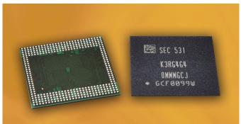
The modules take the same space inside devices as Samsung 6Gb modules, allowing mobile phone makers to either double the device memory within the same space or make smaller phones with 3GB of RAM.
