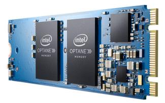
The modules offer limited capacity of only 16 or 32GB, but with latency of under 10 microseconds and peak sequential read speeds reaching 900MB/s Intel claims a performance boost of 28%. The company says storage loads up to 14x faster, while common apps such as Chrome or Outlook load up to 5-6x faster and games can load levels up to 65% faster.
