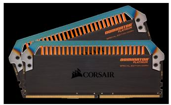
Essentially a fancy version of the previous Dominator Platinum RAM, the Torque model features a top bar heat-treated to look similar to the exhaust manifolds of high-performance engines. It also carries integrated white LEDs for a bit of extra flair. The black aluminium heatsinks get a brushed metal finish, while the cooling fins are in a fetching shade of orange.
