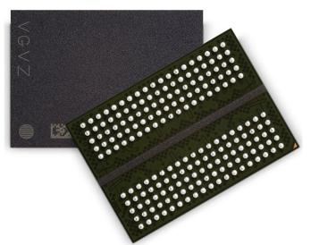
The company first launched "G5X" memory chips at 10Gbps speeds, but now it supplies them in 10, 11 and 12Gdbps, with production focusing on increasing data rates and yields. Currently, the Nvidia Titan Xp GPU uses "Micron's next-gen G5X at 11.4Gbps, which is now in mass production."
