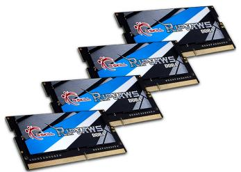
The memory kits ,along the range come in 4 specifications-- DDR4-3800MHz CL18-18-18-38 32GB (4x8GB), DDR4-3600MHz CL16-16-16-36 32GB (4x8GB), DDR4-3200MHz CL16-16-16-36 32GB (4x8GB), and DDR4-3200MHz CL16-16-16-36 64GB (4x16GB). All are based on the Samsung B-die DDR4 ICs, feature XMP 2.0 profiles and require 1.35V.
