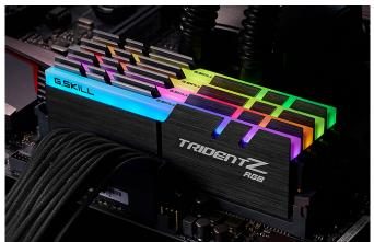
The kits are made using "rigorously hand-binned" Samsung B-die DDR4 IC components, and are rated for DDR4-4000 CL17 17-17-37 at 1.35V, DDR4-4133 CL17 17-17-37 at 1.4V and DDR4-4266 CL17 18-18-38 at 1.45V. The consist of 8GB modules, and come with XMP2.0 SPD profiles to simplify installation on supporting platforms, namely Intel Z370-based motherboards.
